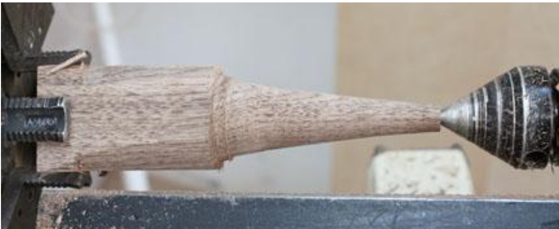
2. Blank turned with tapered cone at end.
