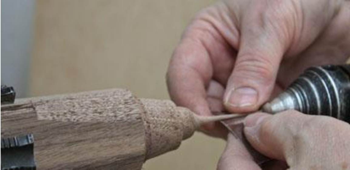
6. Sanding a completed section, supporting the stem to prevent flexing.
