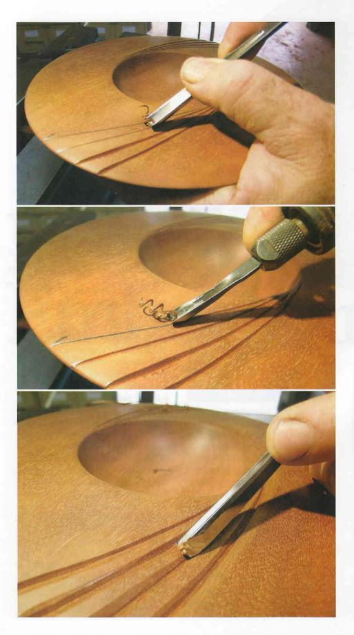
down and rotate the platter in any direction. Another option is to leave the platter on the chuck and then secure the chuck in a bench vise. The main thing is to have the chuck held securely so it does not move during the carving process.
