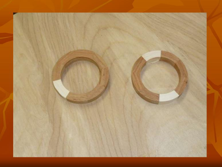
Rings arranged in the correct order for final assembly
