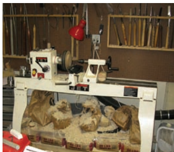
300 lbs. of concrete mix keep the lathe stable.
