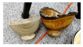
A natural edge bowl represents a special case. The natural edge is delicate, and it's not flat. So a flat faceplate is out of the question. Al had some strategies for holding a natural edge bowl. One is to mount a threaded cylinder, rounded on the end, onto the headstock. Another tactic is to mount a 2-inch square rectangular piece of stock, 10-inches long, into the jaws of a scroll chuck, and
