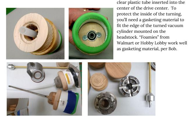
Al says that the vacuum pump is "one of the few safe ways to access the bottom of a bowl." Al prefers to use them with a tailstock in place, and he tries always to cut "towards the center." For the final 1/8-inch, take it off with a chisel. (This works with cross-grain bowls, not end-grain bowls.) Frank mentioned that he always uses a power sander on the base of his turnings. He prefers not to use hand-sanding, which always leaves marks.
