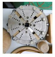
Commercial solutions include the Longworth Chuck. This consists of two plates. One has grooves in it, to adjust to your bowl diameter. The other plate is a backing plate that holds eight nuts with non-mar tips that grasp the turning at eight different points around its diameter. Hint: with the Longworth Chuck, spray WD-40 between the two plates, so they won't stick together. Caution: with the Longworth Chuck, always use tailstock support.
