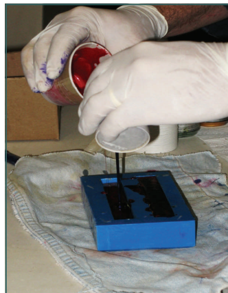
The 2-color resin mix ( www.alumilite.com ) going into the mold
