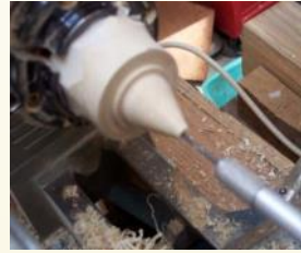
Photo 7. Drilling the 3/32" hole in the cone
