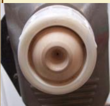
Photo 8. Plug turned to the ball shape
