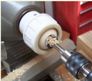
Photo 3. Drilling the 1-1/4" hole about 1/4" deep
