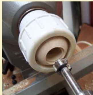
Photo 4. Drilling the 1" hole about 3/4 of the way through the ball
