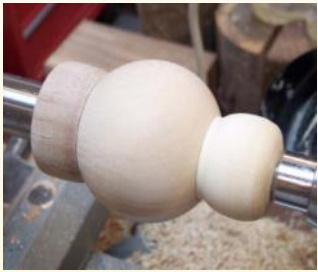
Photo 10. Between centers for Sanding
