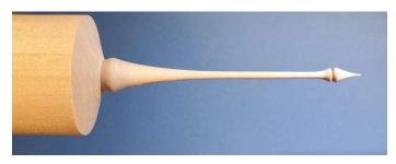
"Sand as you go" is an axiom you must follow, as it is best to sand frequently while a short length of the thin shaft is supported by the thicker, unturned portion to its left. What you *don't* want to do is start sanding when the shaft is 4-inches long, when it would be more vulnerable to whipping or snapping.
