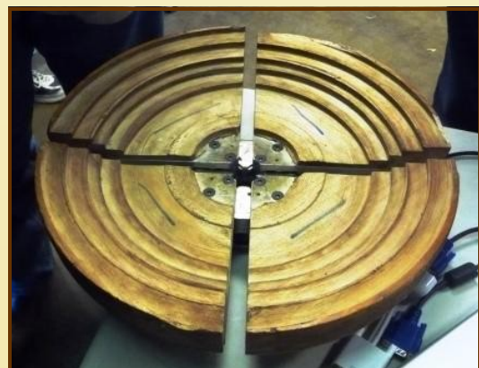
Dale's home made modification to a Cole jaw.
