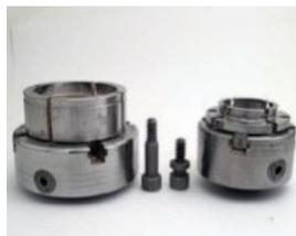
While you can buy a dedicated screw chuck, most scroll chucks come with a woodworm screw. This is a machined screw held within the jaws (Photo 1). A woodworm screw is cylindrical rather than tapered like a typical wood screw and has sharp, deep threads. These threads are designed to bite into the workpiece with a minimum of damage to wood fibers. The screw has a base that fits beneath and against the underside of the jaws to prevent it from being pulled from the chuck.
