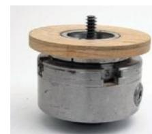
Woodworm screws are not suitable for hollowing projects or other work where the workpiece tends to project out from the chuck toward the tailstock more than about 4" (100mm). Longer projects tend to cause leverage problems that require a stronger holding method than a screw chuck.
