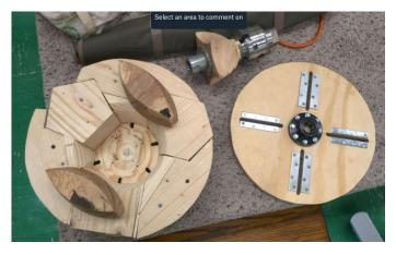
(about 5-inches in diameter) with four, five, and six sides. The 2x6s were then firmly attached to the faceplate using T-nuts and 5/16-inch hex bolts.
