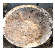
5) Roughed out and ready to dry. The bowl was left approximately 10% of the diameter (15" diameter = 1.5" wall thickness).
