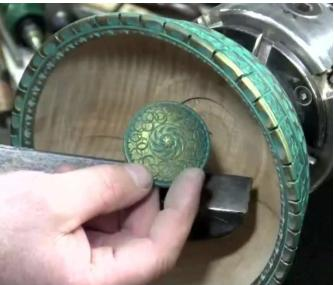
O.D. of the turned button. Lastly, the border around the drilled hole is mated to the curve at the bottom of the bowl. Nick then grabs his airbrush and applies a border of black primer, sealer, green tooth-brush, wipes off the green, puts on the blue nitrile gloves, and applies Bronze and then Gold Gilt with his fingertips.
