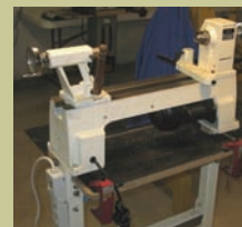
Paul's modified mini lathe. Note the shelf, outlet strip and locking casters
