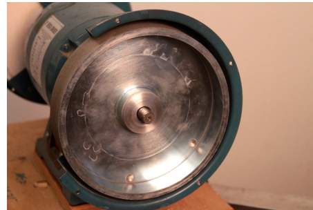
1 1/2 inch wide Optigrind reversed. Plenty of thread left on the shaft. Note holes drilled to balance the wheel.
