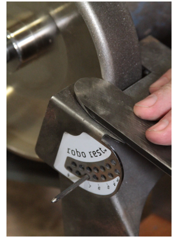
Sharpening a scraper with Radius edge D Way wheel
