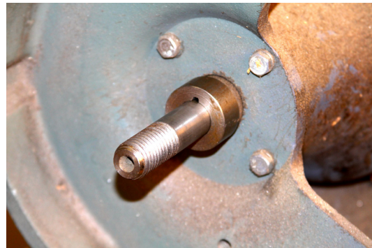
Machined washer with groove / keyway for fitting over the pin on the shaft
