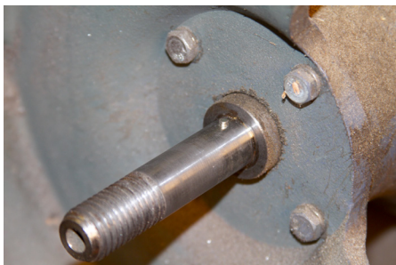
Nib/key on Baldor grinder shaft
