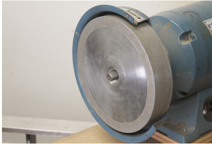
Optigrind with side grind to the outside. It would work with a custom fitted nut that would fit into the recess
