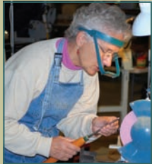
Bonnie puts a good edge on the gouge
