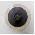
bead on the inner diameter of the facing surface of the blank. Sand. If your beads are good, you should have a perfect torus.
