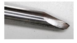
Jason likes to use a gouge with really long, swept-back wings. It saves time. You can use one tool as both a gouge and a skew chisel. His first step with the desert ironwood (DI) blank, after turning it to a cylinder, was to cut a tenon with a taper, and fit it to the top of his bowl opening. Repeatedly. Once the tenon on the DI was cut to his satisfaction, he cut a mortise in the poplar holding jig. There's a lot of trial and fit here.
