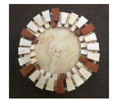
After the first layer of segments has been glued into place, wait 10 or 15 minutes for the glue to dry. You will need to turn on the lathe to flatten this ring so it is a flush surface upon which the next ring pieces will be glued. To flatten, use a round-nosed scraper (gently), or put a piece of sandpaper on a sanding block and gently touch the surface with
