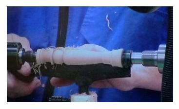
exercise in making beads, and in the case of the top hat, a shallow cove. The bead for the head should be close to a sphere. Too pointy? Then go back to the center of the bead and reduce the high point with your spindle gouge, using a back-and-forth body movement to render the head curve uniform.
