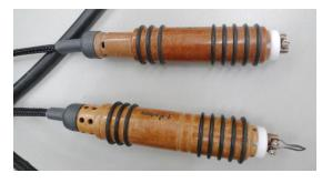
Vesery's surface texturing techniques include rotary tools from Mastercarver, which are similar to a Foredom tool, but less expensive. The basic Mastercarver model with foot pedal, which he uses, is available from <u>www.woodcarverssupply.com</u> in Florida. You could also use a Wecheer (available from Woodcraft) or a Dremel rotary tool, but you get tired holding the heavier Dremel
