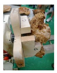
The challenge with turning a bowl from a burl is figuring out how to build a sturdy jig to hold the burl in the lathe. Roger had a rather elaborate one already attached to the headstock, ready to be turned.
