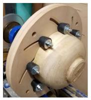
11.5-inch outside diameter with 8.5-inch maximum 4.0-inch minimum grip range Latex gripers. Face plate with 1-inch-diameter 8 threads per inch or a face plate to fit your lathe, call with your details. Outside diameter can be changed to fit your lathe. 24, 22, 16 inch available.
