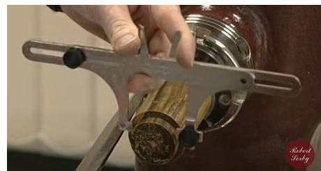
Turning the external thread diameter
