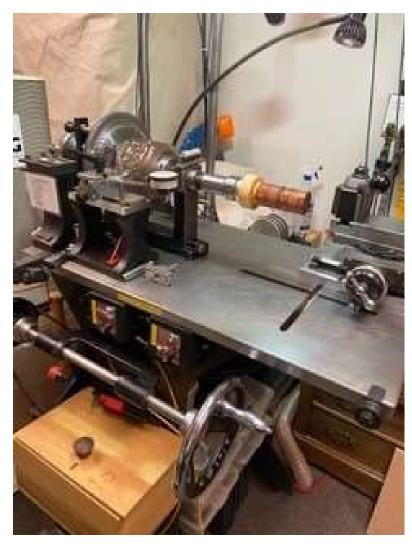
sizes, very precisely. With the drilling frame held perpendicular to the workpiece, a different set of carbide cutters can produce "pearls" (little raised dots) on the side of the workpiece, located precisely around its circumference at intervals of the operator's choosing.
