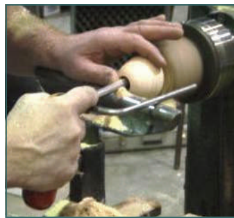
Hollowing with the Don Derry Tool
