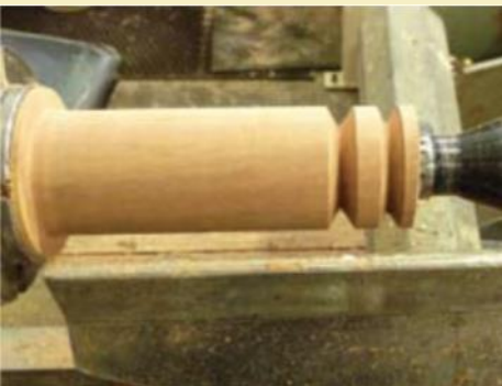
Figure 2. Two V-cuts have been made near the tailstock. The space in between the cuts will define the knob on the end for teething.
