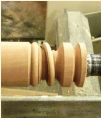
Figure 5. Starting the second loose ring.
