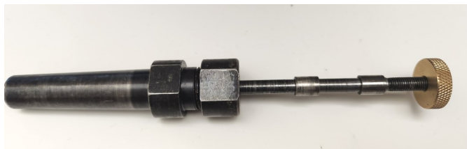
Professional pen mandrel (Shown with two slimline bushings)
